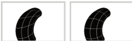
The left picture represents a non-stretched projection of the grid on the bend, in such a way that the cell size of the grid varies when projected on the bend. The right picture represents a stretched projection of the grid on the bend, in such a way that the cell size on the bend is kept constant. In that case a white line is visible on the grid. When you click on the picture of the band, it will change to the other representation.
